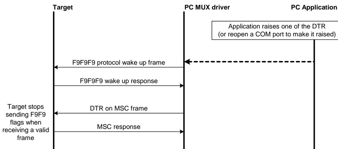
*Note:* If the valid frame is a DATA frame, the embedded module does not detect any DTR change and sleeps on again with the PSC frame.
