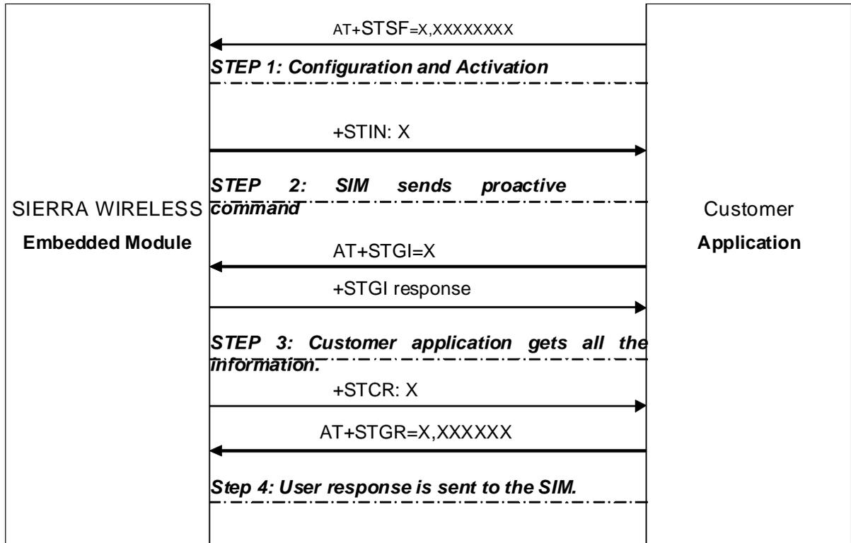
On the first step, the customer application informs the Sierra Wireless product which facilities are supported. This operation is performed with the +STSF (SIM ToolKit Set Facilities) command, which also allows to activate or deactivate the SIM ToolKit functionality.
