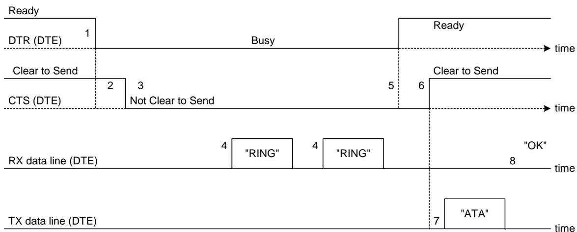
1: The application (DTE) drops its DTR to indicate to DCE a busy state
